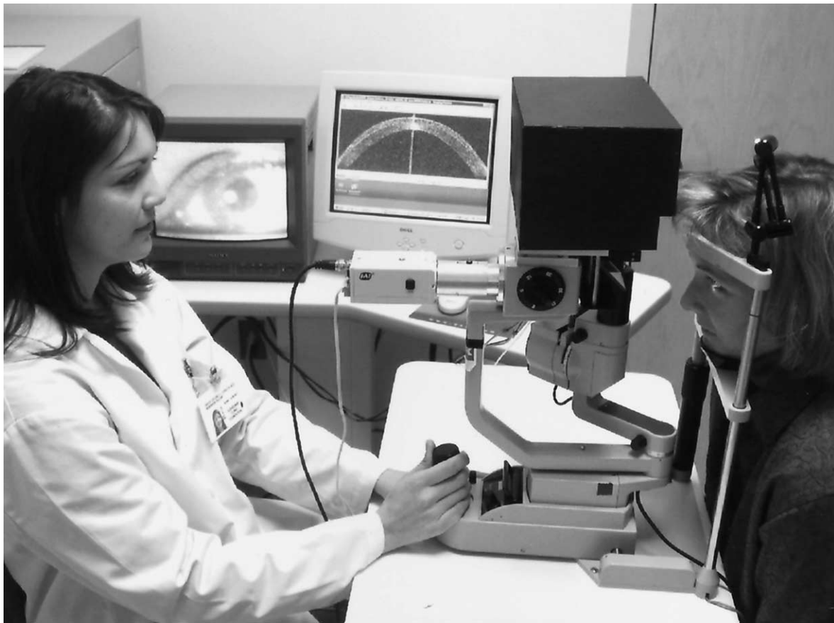
Figure 1. One of the authors (MRC) demonstrating the use of the corneal and anterior segment optical coherence tomography (OCT) prototype. The OCT hardware is contained within the black box on top of the slit lamp. The OCT image is displayed on the monitor on the right, and the charge-coupled device video is on the monitor on the left.
